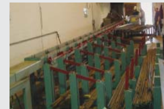
Stock is conveyed indoors to shear and sent to automatic and manual bending downstream.
