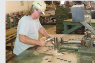
Stock is conveyed indoors to shear and sent to automatic and manual bending downstream.
