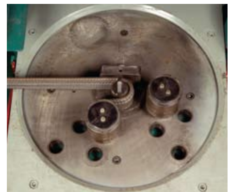
Handles column offset bars easily with optional tooling
