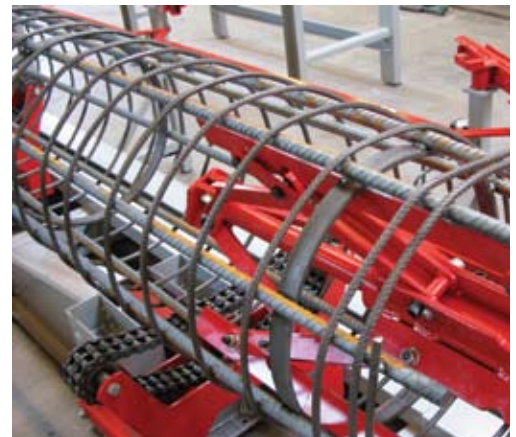
Innovative spindle arm securely holds and spins cage.
