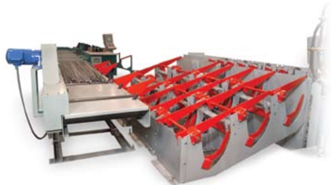
LiftRoll runout conveyor being elevated and bars are conveyed downstream to other operations
