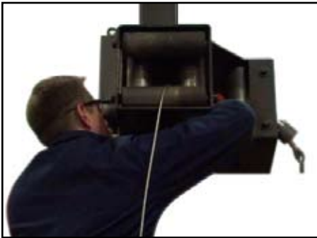
Operator feeds bar guide and winch wire through cradle carrier guide.
