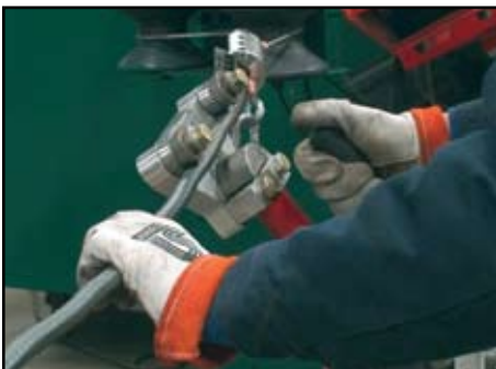
Operator uses optional hand-held straightener to straighten end of bar while winch holds bar in place. Then operator guides bar into the machine.
