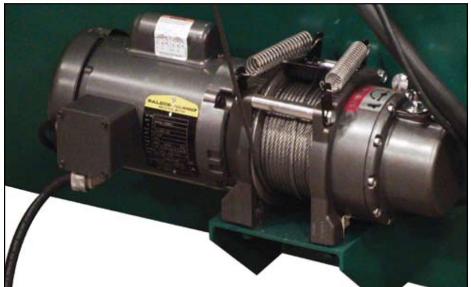
Winch pulls bar toward machine.
