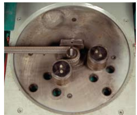
Handles column offset bars easily with optional tooling
