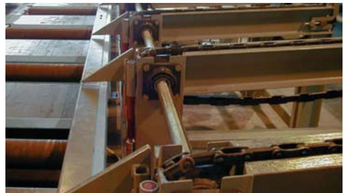
Horizontal Chain Drag Loading System Optional
