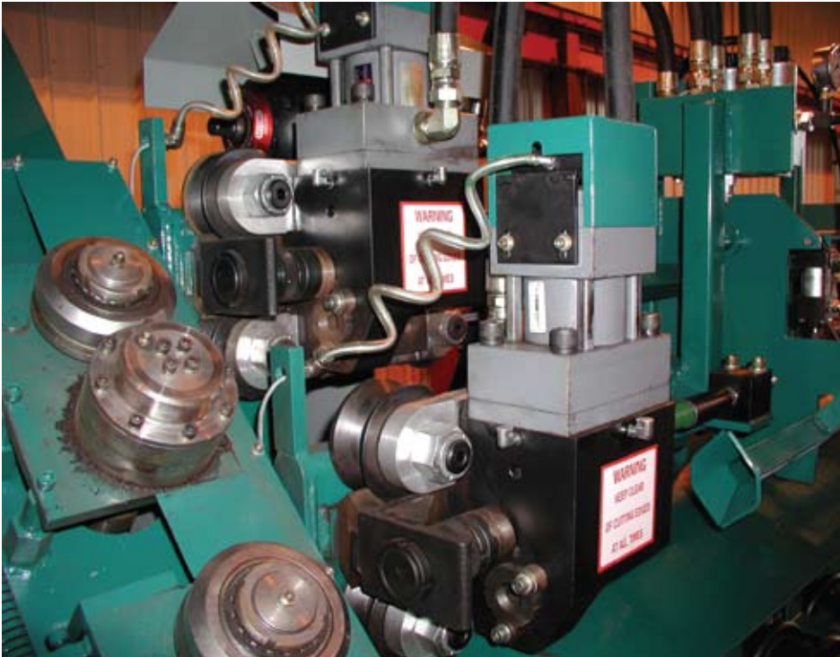
Heavy duty flying shears cut up to #5 (16mm) rebar at 360 ft./min. (110m/min.)
