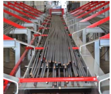
Innovative preload arms allow bars to be loaded while others are being sheared.
