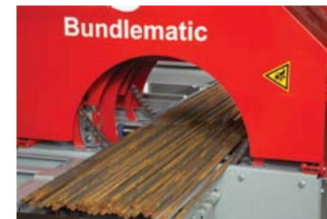
The BundleMatic gathers loose rebar up in a tight bundle.
