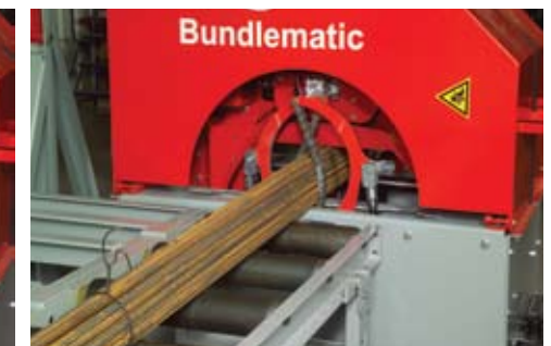
The bundle is conveyed down and then wrapped at whatever interval is needed.
