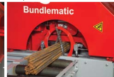
The feed wire spool is lowered on top of the bundle and then spun around and twisted.
