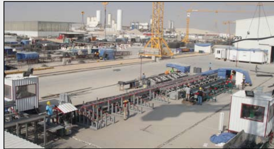
Two KRB Standard Shearlines with bar transfers to double benders operate on the university project site.
