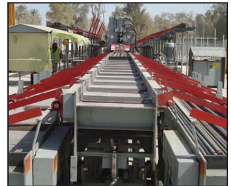
KRB Standard Shearline with conveyors to bending stations down stream.
