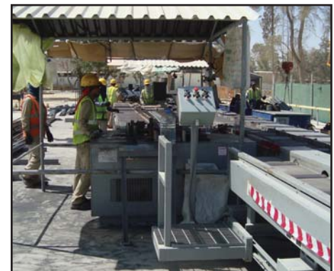
KRB #18 Bender is a heavy duty bender for large bar sizes.
